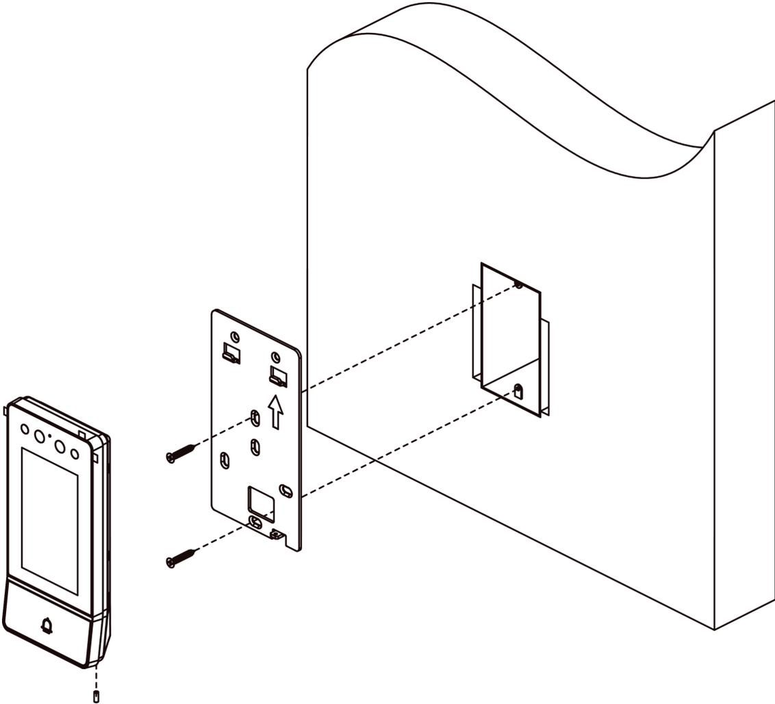
Figure 3-4 Flush Mounting
