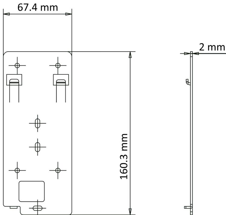
**Figure 3-1 Installation Plate**
