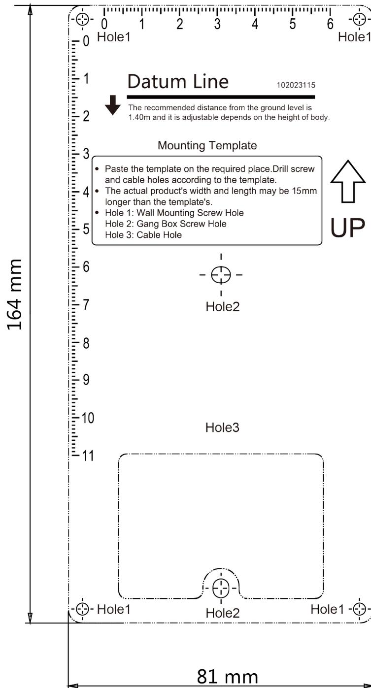
**Figure 3-2 Mounting Template**
